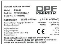
V<sub>out(max)</sub> and V<sub>out(min)</sub> are defined by the slope of each sensor. This means, the output is capable to be between 0.5V and 4.5V; the actual signal output range depends on the calibration value and the torque range.
